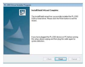
Click "Finish" to complete the installation, now you can plug the converter to the USB port of the computer.
